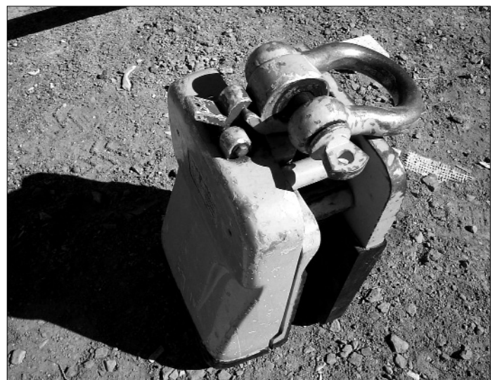
External Lewis: Gravity-clamp Slab Lifter.
