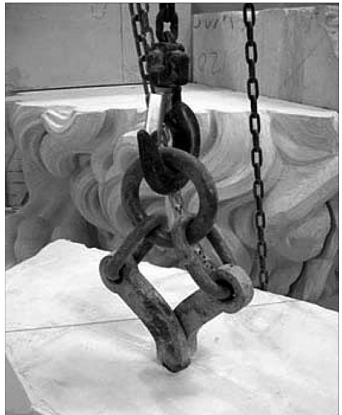
Close up showing Lewis Pins and demonstrating how lifting ring transfers a sideways pressure to make inserted prongs grip the side of the hole.
